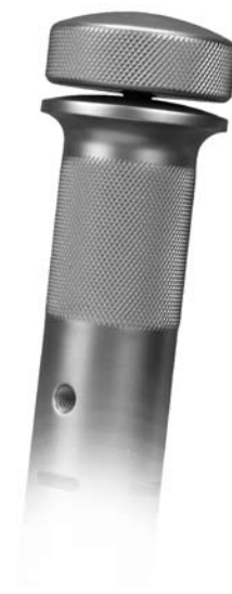
Fig. 14b Strike plate not fully seated against impactor plate
