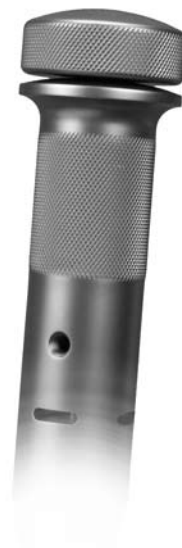
Fig. 14a Strike plate fully seated against impactor plate
