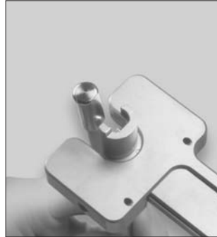
9. The tibial component is loaded onto the tibial target frame.
