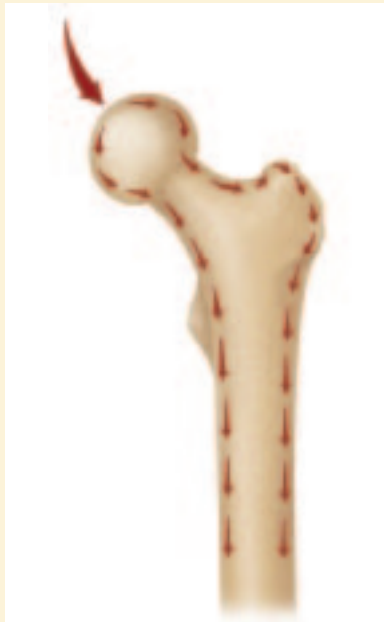
Load transfer patterns for the natural femur
