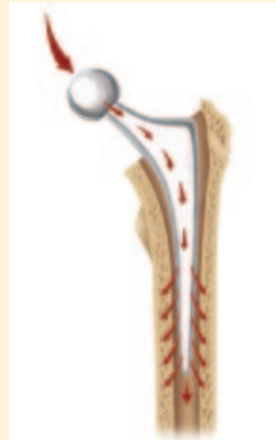
Load transfer pattern from conventional dual taper highly-polished cemented stems
