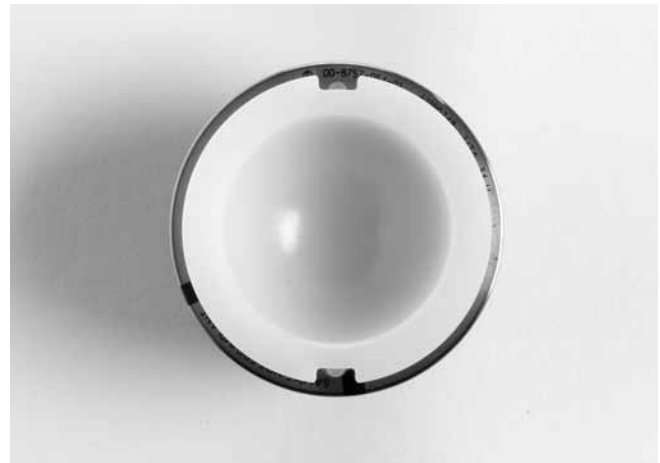
Fig. 8 Smaller size Liner with cut-outs assembled into the Shell.
